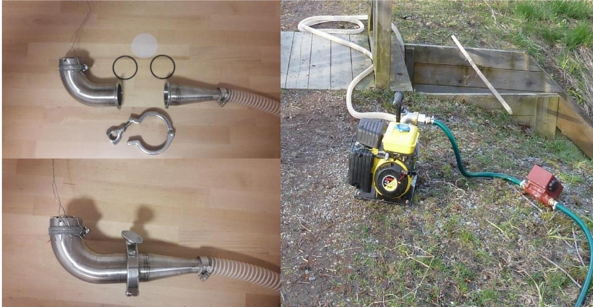
Figur 1. Equipment used for sampling of microplastics. On the left hand side: filter holder consisting of stainless steel pipes with a chamfer for gaskets, a nylon filter and a corresponding clamp. The filter holder was designed with a bend only to improve sampling in very shallow waters and to decrease the risk of sediments being filtered. To the right is the gasoline driven water pump connected to the filter holder and a red volumeter.
