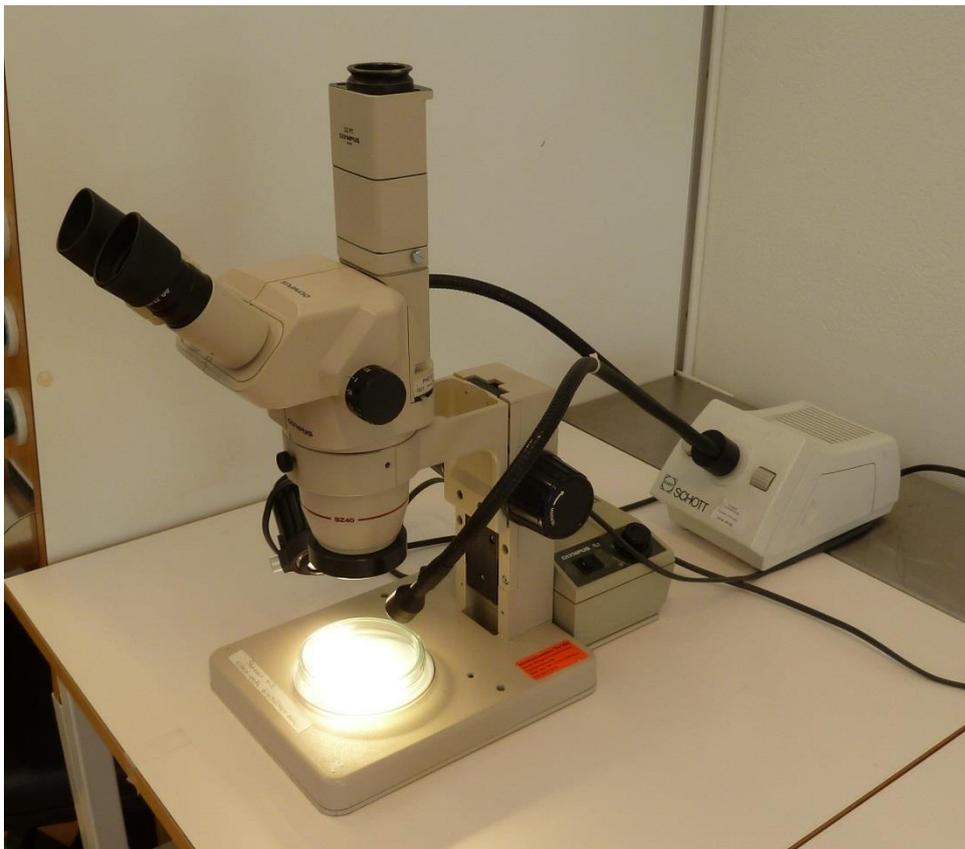
Figur 2. Stereo-microscope and petri dish containing a filter.
